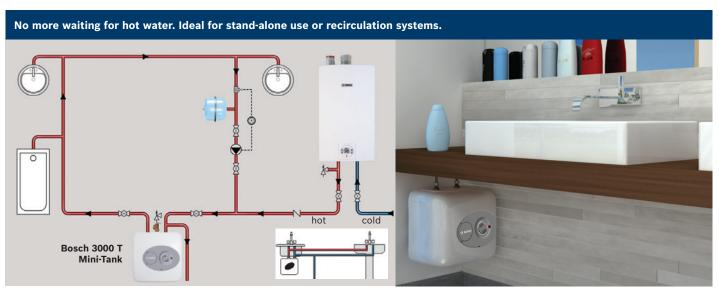
Relief valve is required; however it is not shown in above photo for clarity.
