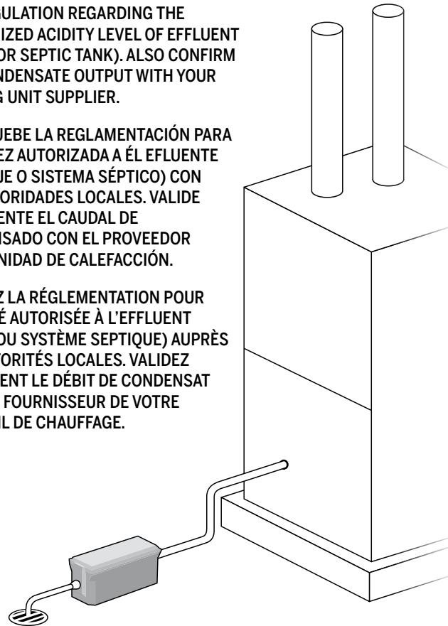
CondenSAFE is provided with connectors for hard piping (PVC). If you wish to use flexible hose, you can obtain the #CSHK kit at your local dealer.
