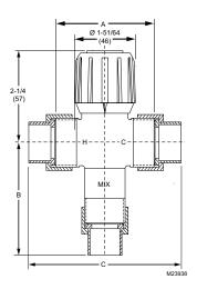
Fig. 1. Dimension Diagram.
