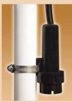
The compact level sensor detects the liquid level in the tank and sends a signal to the IP panel which displays this level in inches or centimeters for easier monitoring of the system. Pump activation and alarm levels can be adjusted using the panel touch pad - eliminating the need to go into the tank for manual adjustment.
