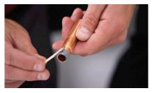
**6.** Working quickly, apply epoxy completely to outside of reduced end of repair adapter.
