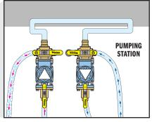
Configure the valves to isolate the building loop. Connect a source to the outer port on one valve in the ground loop and a drain hose to the other. Air in the ground loop will be forced out of the purging port by the incoming water.
