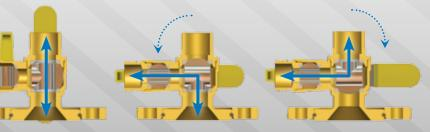
**MULTI-FUNCTION DRAIN - Purges Before or After Pump**
