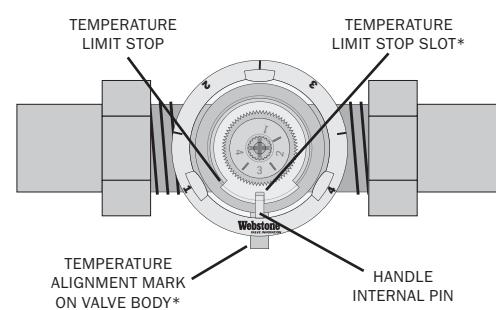
If desired, the temperature setting can be fixed on the Webstone TMV by locking the handle in place:
