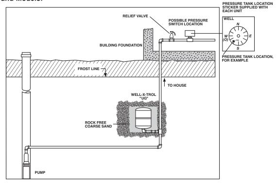
**All Well-X-Trol Underground Tanks** are designed for direct burial and must be installed **in the vertical position only**. To eliminate danger of freezing, tank should be buried below the frost line.
