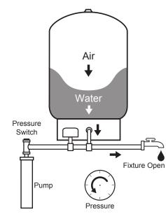
The amount of water delivered between pump cycles is called drawdown. The larger the well tank, the greater the drawdown capacity, the less the pump needs to run. This saves energy and
