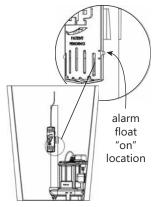
mark on the side of the float housing, the alarm will activate. Alternately, a cup of water can be used to confirm float operation. Raise the cup of water up to the float, and submerse the float past the bump on the right. This will trigger the alarm.
