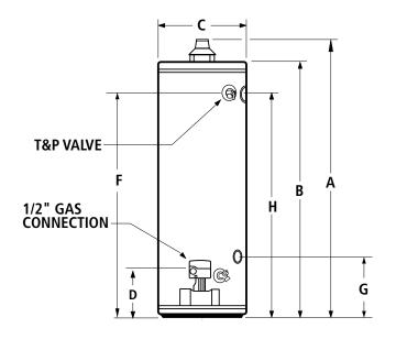
Maximum Hydrostatic Working Pressure: 150 PSI
