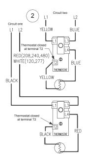
When either thermostat is satisfied, it will open at terminal T2, interrupting current flow through the corresponding element. As both thermostats satisfy, the system will be in stand-by mode waiting for the next call for heat. Thermostats will operate independent of each other.
