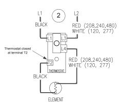
When the thermostat is satisfied, it opens at terminal T2 interrupting current flow through the element. System is now in stand-by mode, waiting for the next call for heat.
