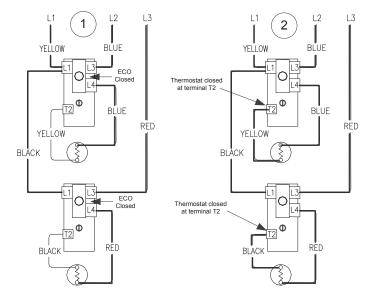
When either thermostat is satisfied, it will open at terminal T2, interrupting current flow through the corresponding element. As both thermostats satisfy, the system will be in stand-by mode waiting for the next call for heat. Thermostats will operate independent of the other.
