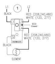
2 Tank is cold therefore thermostat is closed at terminal T2 (calling for heat). This completes the circuit and allows current to flow through the element.
