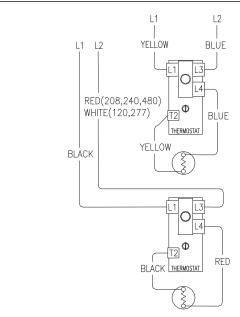
Reference 4 Wire, Simultaneous, Single Phase Wiring diagram.
