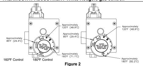
The thermostat dial is set to its lowest temperature setting when shipped from the factory.
