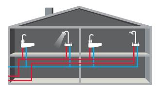
What is a comfort hot water recirculation pump? A hot water recirculation pump is designed for recirculation of domestic hot water in single family homes with dedicated hot water return piping.
