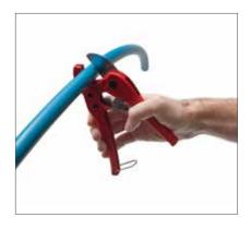
**1.** Square cut PEX pipe 90 degrees to pipe length.
