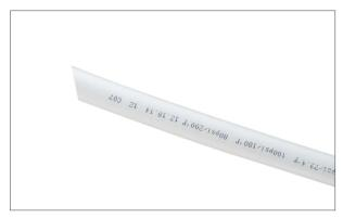
Tube not cut squarely – ring and tube need to be mated perfectly and installed fully over F1960 barb for a viable seal.
