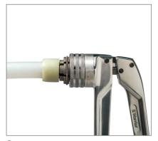
3. Using tube expander, expand sleeve fully. Repeat expansions, rotating expander 1/8-turn between expansions. Note: To limit the amount of time for tube compression onto fitting in cold environments, expand the tube/sleeve slowly and only enough to fully insert the fitting. Keeping sleeves warm will speed retraction and inhibit unequal expansion.
