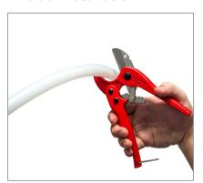
1. Cut tube at 90-degrees. Do not crush OD of tubing with cutters. Hint: Slightly rotate cutter during blade engagement.
