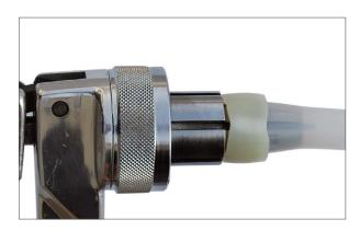
Ring must be kept around 55°F or greater to assure expansion is uniform. Remove any expanded ring that displays unequal expansion. Failure to rotate tool inside tubing may cause unequal expansion.
