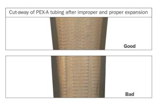
Leak path. Expansion did not rotate between multiple expansions, leaving a groove or leak path past the fitting barb. Expansion made with a defective expansion head.
