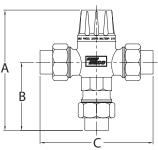
**5000 Series Mixing Valve Dimensions** Dimensions for reference only
