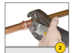
Using approved press tool and jaw of the correct size, open the jaw and place over the bead of the fitting or valve at a 90 degree angle to the tube centerline.
