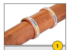
Insert the tube into the fitting or valve with twisting motion until it meets tube stop AND insertion depth mark. Wetting the tube, fitting or valve with clean water may reduce insertion force.
