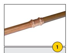
Insert the tube into the fitting or valve with twisting motion until it meets tube stop AND insertion depth mark. Wetting the tube, fitting or valve with clean water may reduce insertion force.
