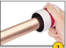
Remove internal and external burrs at tube ends using fine tooth file or commercially available de-burring tools.
