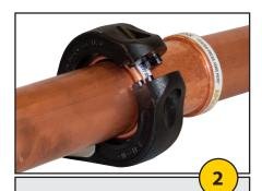
Using approved press tool and ring, sling, chain of the correct size, open the ring, sling or chain and place over the bead of the fitting or valve at a 90 degree angle to the tube centerline.
