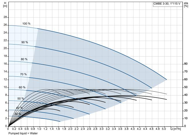
Liquid temperature during operation = 20 °C
