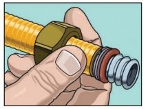
2. Place Retainer and Slide Ring in the fourth valley. Place o-ring in third valley. Ensure gasket is in fitting.
