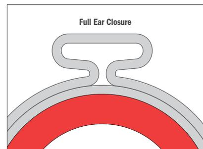
Check ratchet pincer tool calibration with a GO/NO-GO gauge daily. Refer to tool manufacturer's instructions for calibration procedures.
