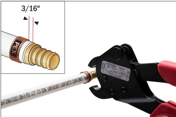
3. Position ring over sealing barbs of the fitting. The ring should be positioned approximately 3/16" from the end of the tube.
