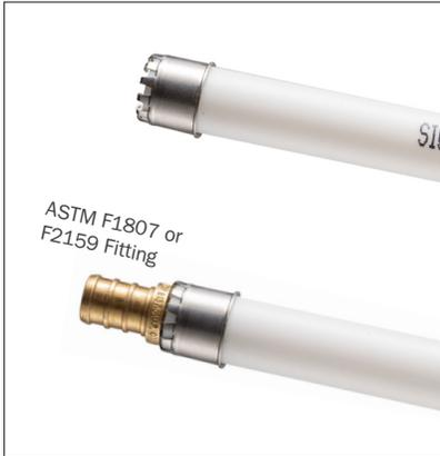
1. Cut tube at 90-degrees. Install V-Sleeve onto OD of tube with notched side towards tube end. Install fitting fully into tube. Visually confirm tube is fully inserted through notches.
