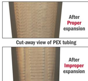
No rotation between expansions, or defective expansion head leaving a groove as a potential leak path.
