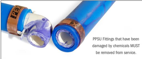
PPSU Fittings that have been damaged by chemicals MUST be removed from service.
