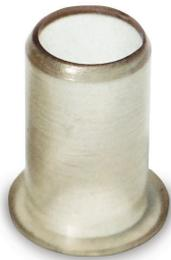
Stainless Steel or PPSU PEX inserts must be used when a supply fixture valve will be pushed or compressed onto PEX tube. ASSE 1061 push-fit fittings for use on plastic tubing must use an insert sized appropriately to the tube type ID.
