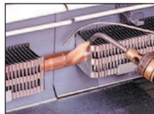
**Vented return bend**. Special 180° bend aligns return line perfectly with half-moon cutouts in support brackets. A 1/8" threaded tapping permits easy installation of air vent, can also serve as a drain.
