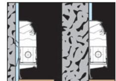
**Snap-on, hinged accessories** swing up for easy access to air vents and heating element or for removal of the front panel— even when wall material covers the accessory top. Precision piano hinges last for years.
